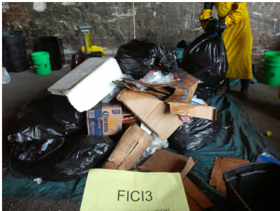
Sample FICI3 is ~ 200 pounds of waste from the tipped load. Sample Coordinator stays with the sort staff and Crew Chief until sample is pulled and documented. Placard stay on sample until it is processed (sorted and weighed)
