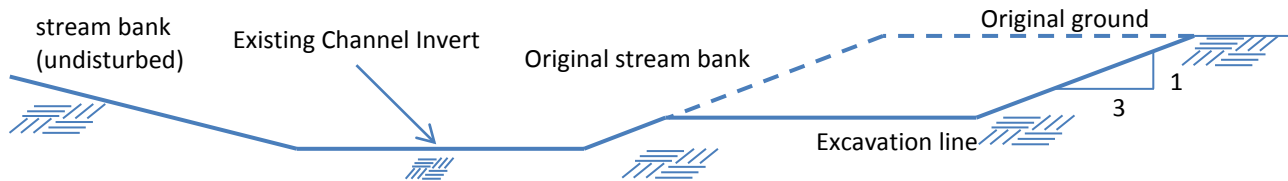
Figure 7.3: Typical Channel Modification Cross Section
