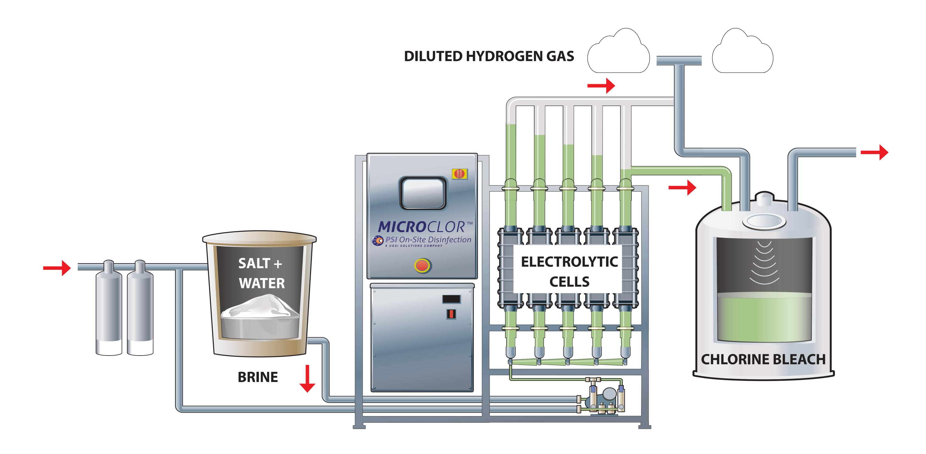
NaCl + H<sub>2</sub>O + Electricity = NaOCl + H<sub>2</sub>
