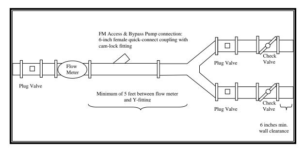
Meter/Valve vault will require a gravity drain to the wet well (with check valve) or a small sump pump.
