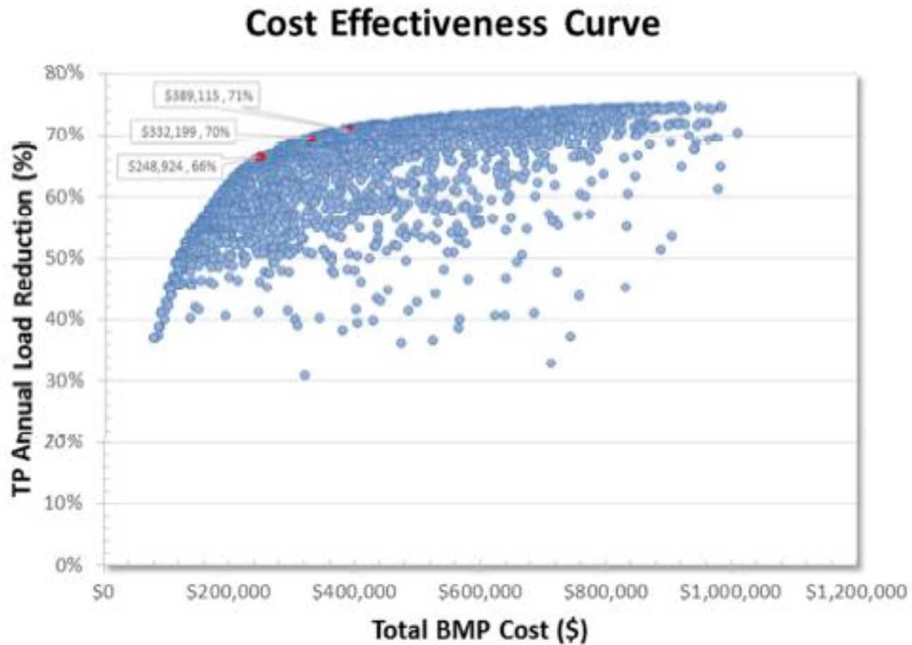
Figure 31. Cost effectiveness curve for potential bmp combinations.
