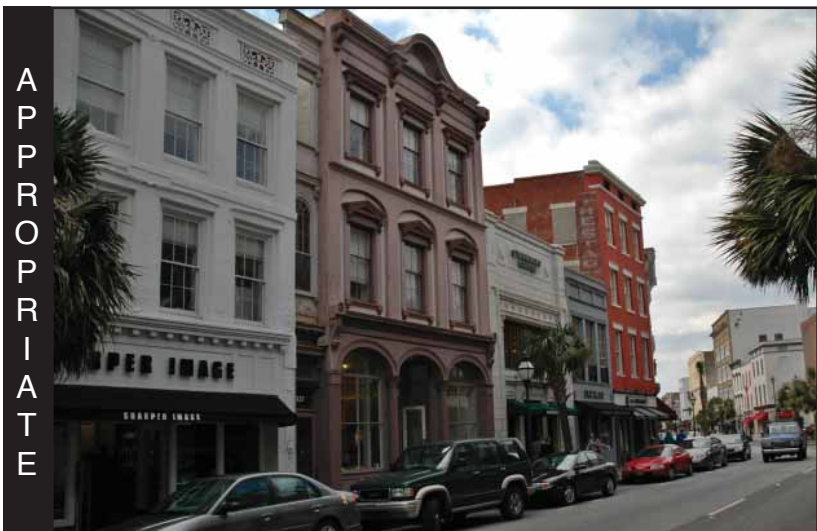
Photo 11.10—Dimensional cornice treatments over upper level decks as shown in photos 21.3 and 21.4 help to create visual interest along the roof line of this street facade. Ground level awnings help accentuate individual framed windows and high-light entrances.
