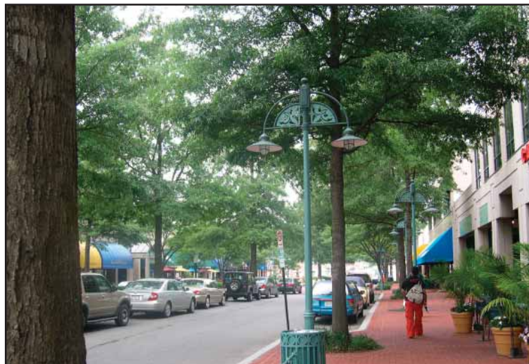
Photo 7.5—On-street parking serves as a buffer between the pedestrian and adjacent lanes of traffic.
