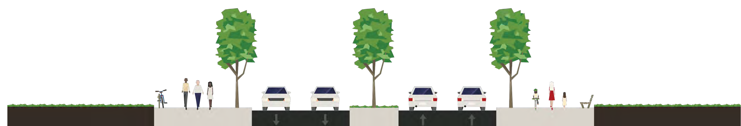
Consolidated Cross-Section - Median Condition
