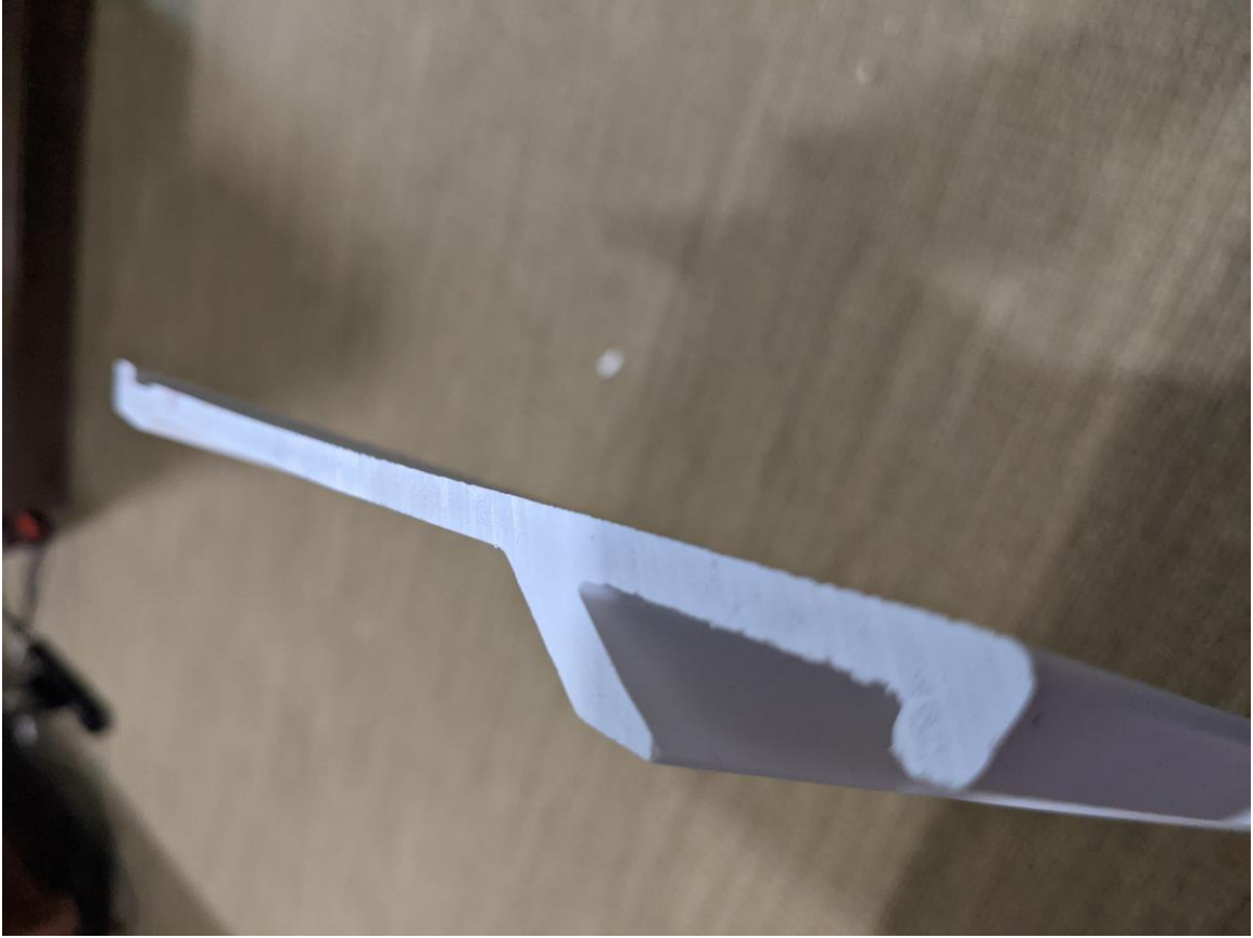
Edge of the proposed siding. The top is the front face of the material.
