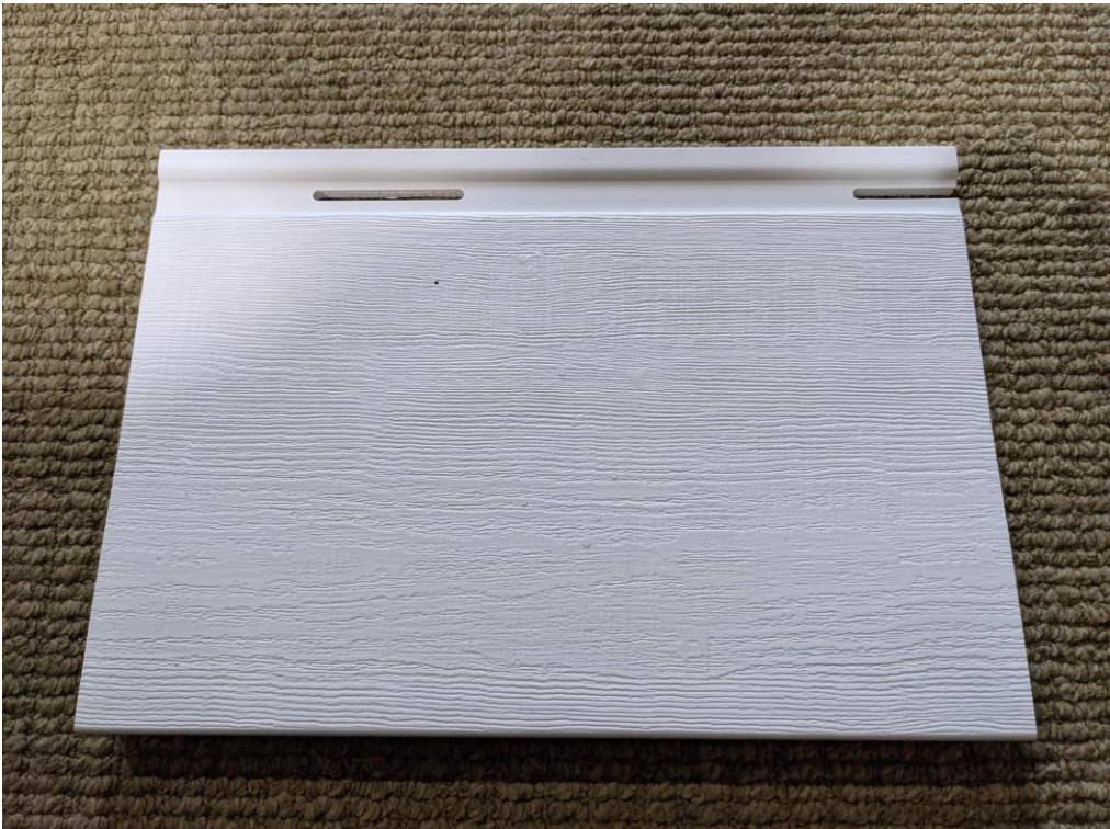
Sample of proposed material. The tab at the top shows that it is installed in a similar manner to vinyl siding, which is not an approved material.
