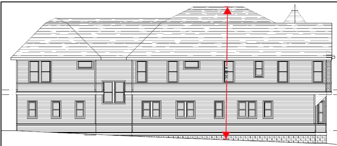
Figure 3. Left side elevation (north). Height at arrow is thirty-six feet, six inches (36'6") tall.
