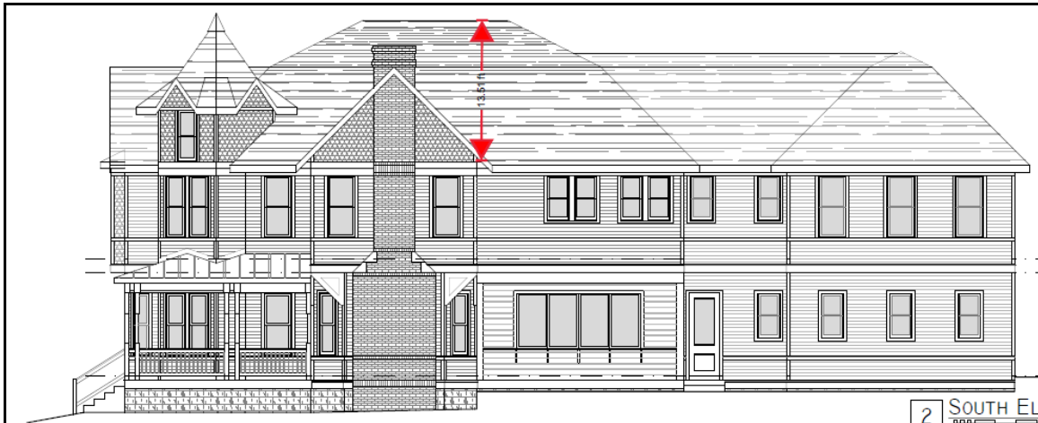
Figure 3. South side elevation. Arrow indicated 13'6" height of roof.
