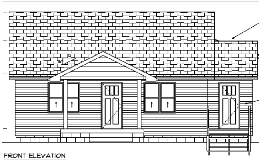
Figure 3. Front elevation, showing side addition
