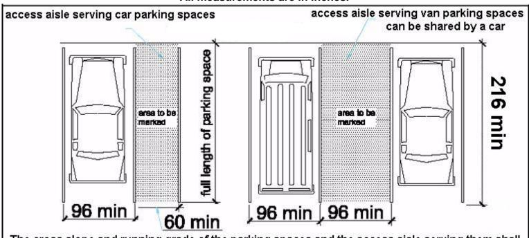
The cross slope and running grade of the parking spaces and the access aisle serving them shall not exceed 2% (1/4" per foot) in any direction.
