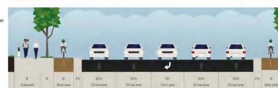
\*Final build out may deviate lane assignments based on approved TIS Final street design will be coordinated with Planning and Public Works based upon the approved TIS and shall include a planting area, sidewalks, and bikeway facilities
